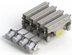
NT series machine's vibration table is equipped with 4 synchronized servomotors. The vibration table is supported by high-strength rubber buffers to maintain an even vibration across the table. Fully automatic control system allows to adjust frequency, power and amplitude of pre-vibration and main vibration at any given moment without
