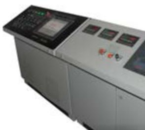
Production process is controlled by one operator via control panel equipped with a LCD touchscreen, which displays all parts of the system in individual pictures. Upon touching the chosen unit the menu appears showing current operating mode and preset parameters. The parameters can be changed in real-time without stopping the production. The software has user-friendly interface while all information is written in customer's preferred language.
