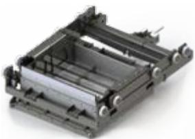
Hydraulically driven agitator grid, mounted inside the base concrete filling box, ensures fast and even filling of all mould cavities. As a result all concrete products have the same density and dimensions.
